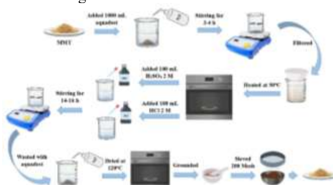
Figure 2. Illustration of MMT activation
